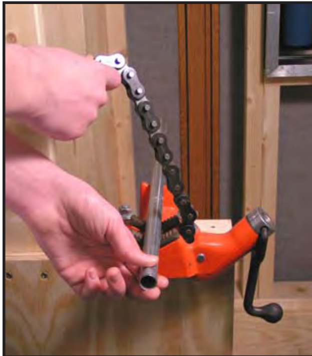
Placing the Pipe in the Chain Vise
